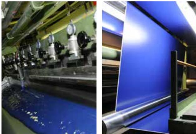
**The applied FLEXOTHANE® coating formula is of key importance. We use an European origin high grade hydrolysis resistant PUR.** The European standard EN 343 class 3 (meaning minimum 130 cm of waterproofness) is applying a range of pre-treatments to the fabric after which we still need 130 cm waterhead. As received we easily have waterproofness results of >8m (or 800 cm).
